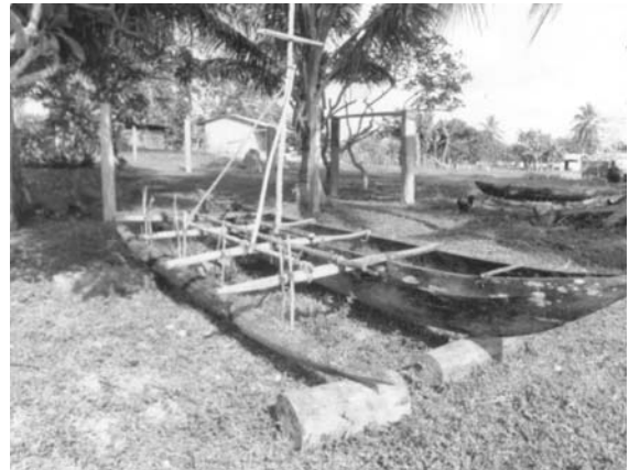
Seafaring in the Polynesian Outliers. Fig. 7 Anutan outrigger canoe of tovi type, on beach in Russell Islands. The canoe is rigged with a lantern holder for catching flying fish at night.
